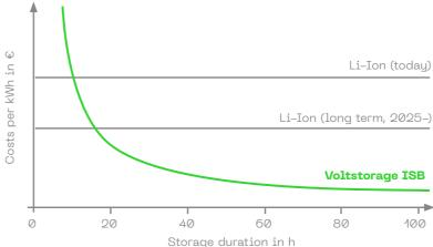
With iron salt battery technology, we are relying on an iron-based storage medium - and thus on one of the most abundant raw materials in the world. The use of ecological materials allows the storage technology to be scaled according to the given needs, resulting in economies of scale. In addition, thanks to the CO<sub>2</sub>-saving technology, power from renewable energies can be stored in a sustainable manner, thus making a double contribution to combating climate change.
